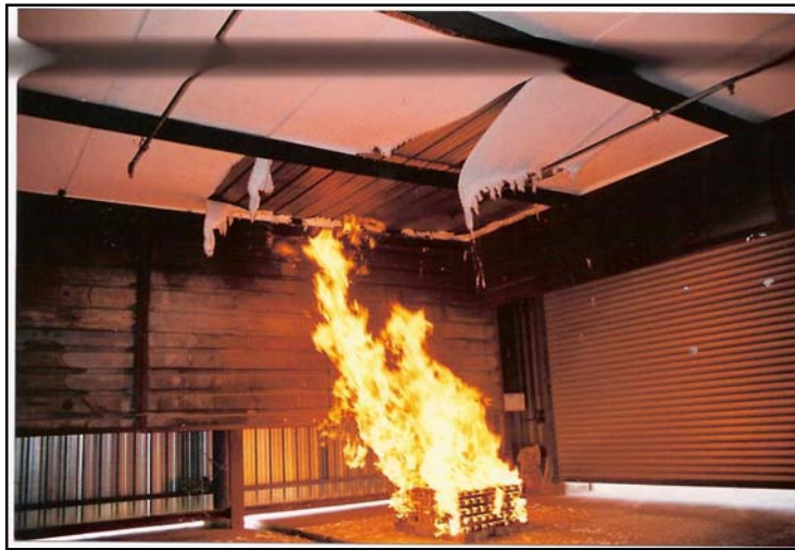
Figure B2-2: Installation damaged in area above fire source (t = 5 min)
