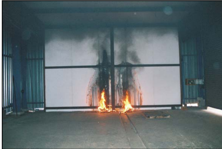
Figure B3-3: Starter packs collapsed against installation with some fallen material burning between bottom purlin and IBR sheeting (t = 19 min)
