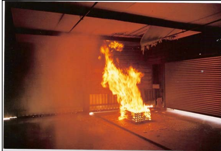
Figure B2-3: First sprinkler activated and operating unhindered (t = 7 min 30 s)
