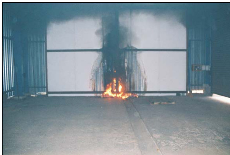
Figure B3-4: Limited flaming along vertical support element (t = 22 min), which seized at t = 24 min)
