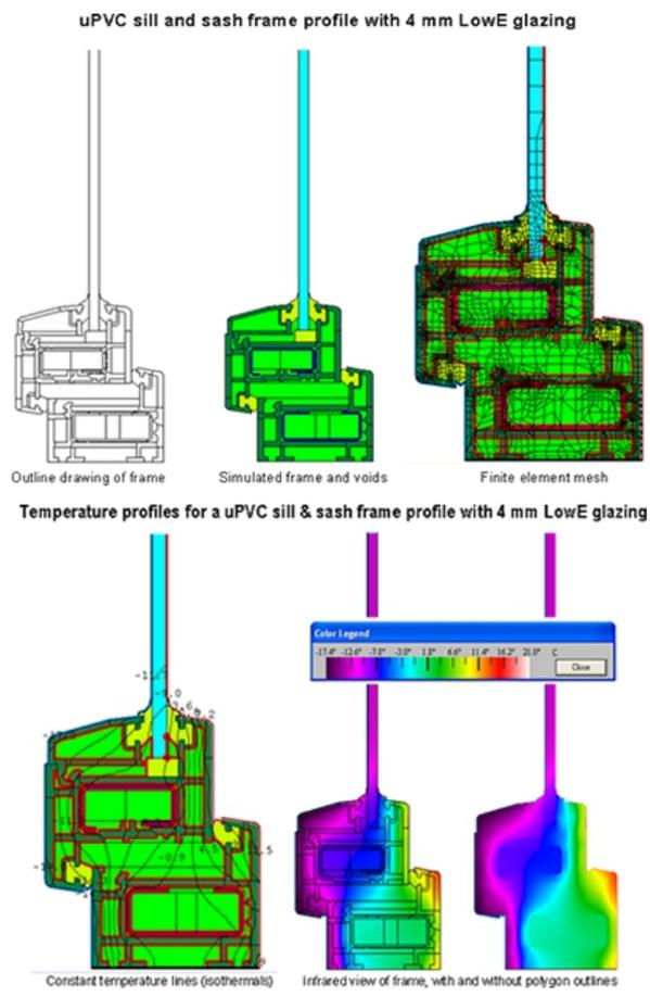
The THERM Program is a two-dimensional (2-D) finite element program for calculating heat transfer in fenestration systems and other building envelope constructions. In addition to conduction heat transfer, the program also handles detailed radiation heat transfer, based on view factors. It also incorporates convection heat transfer modeling in glazing cavities.
