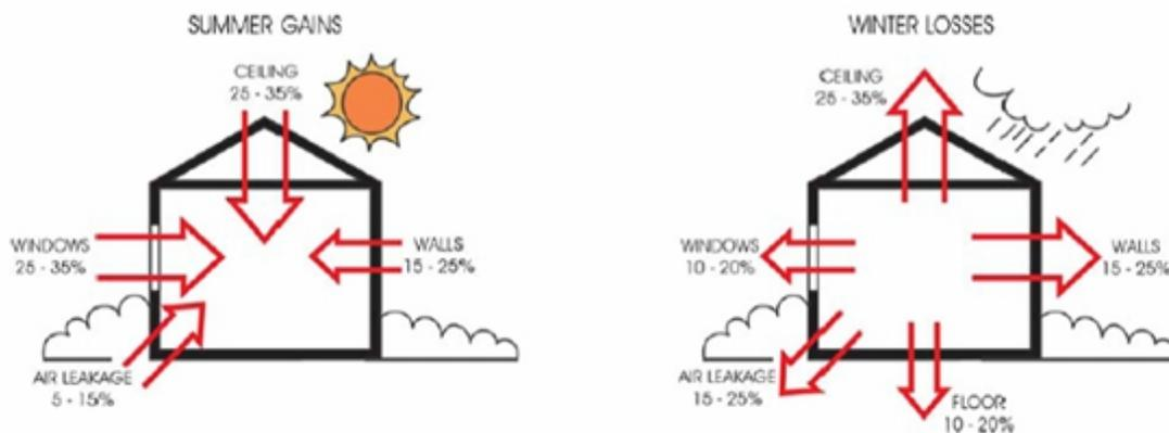
The term 'insulation' refers to materials or a combination thereof which provide resistance to heat flow.
